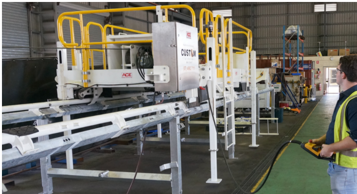
The innovative custom-designed Mobile Bolting Working Platform
