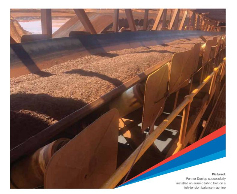
"One of the key drivers to the Kordflex® success was the innovative highly specialised method of joining the conveyor belt together. Kordflex® adopts a single ply construction and hence traditional methods of joining were not applicable," Lindgren said.
